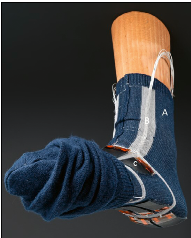
Figure 1: Prototype of the PressureTrack sock made of SMOOLS (A) with the sensors (B) and corresponding cable ducts (C). At the current stage of the prototype, a second sock is worn over the sensor-equipped sock. (Fraunhofer ISC)
