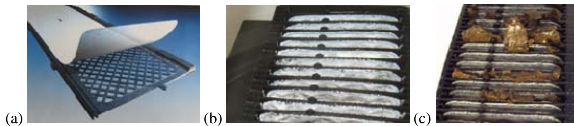
Figure 1: view of a single membrane plate (a), the top of a clean plate and frame module (b) and a blocked membrane module (c)
